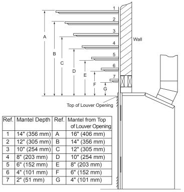
Figure 6 - Clearances for Combustible Mantels
